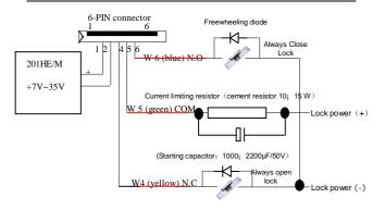
A capacitor with low series resistance is required, for it can release peak value current required by starting. For example, if the lock is started to lock on in case of +12V, when the resistor is connected, favorable locking status can be maintained when the voltage is reduced to about +8V.
