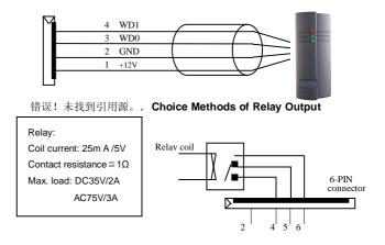
Definitions of lead wires: 2: GND; 4: N.C; 5 COM; 6 N.
