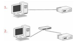
The PC that is connected directly to the NVR (or within the same local area network) should receive an IP from the NVR. Simply access the NVR from your web browser with its IP address
