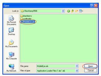
You will now return to the Application Loader screen. From here you should see "MobileEye" now listed with Install under the Action column (shown as follows) if the installation is successful.
