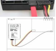
Your HDD should be installed inside the DVR. Please connect the HDD in the standard way, screwing the HDD into the HDD brackets or DVR base. All necessary cables are delivered with the DVR. Use instructions that came together with the hard drive for exact wiring and installation. Please connect the power cable to the appropriate socket, and the data cables to their corresponding connectors.
