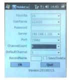
In the following screen, input the User Name, Password, Server (IP address for your DVR) and Port (default 10510). Next, choose the channel Count for streaming data from the drop-down menu and choose the Default Channel when connecting. Choose a Record Name for your favorite files.
